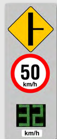
GR33CL Sign 700mm x 2250mm W002R Diamond with 600mm Dia. Speed Limit Roundel
